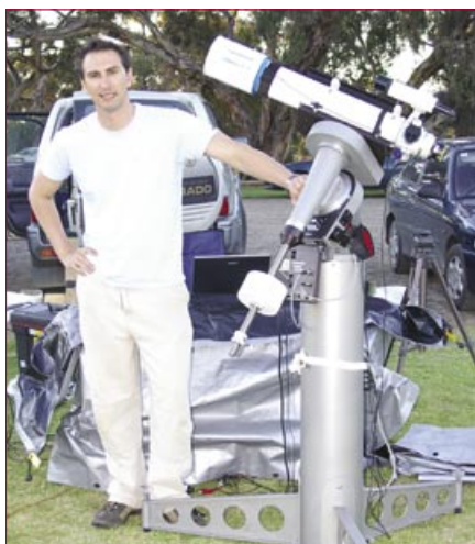
Chris Venter and his Takahashi FS-102 on a Mountain Instruments MI-250 and custom-made 8" stainless steel pier.
